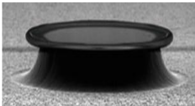
Figure 6: SEM image of a silica microdisc [36].
