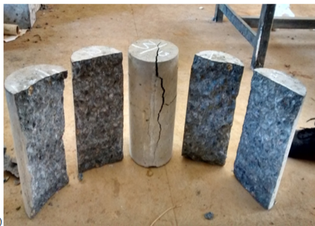
Figure 6: 1.5% fibre-added concrete cylinders after split tensile test.
