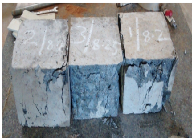
Figure 5: 1.5% fibre-added concrete cubes after compressive strength tests.
