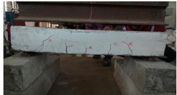
**Figure 4: Cracked beam**
