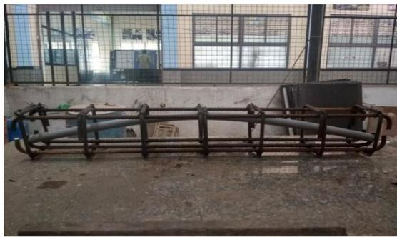
**Figure 1: Arch action in placing of reinforcement**
