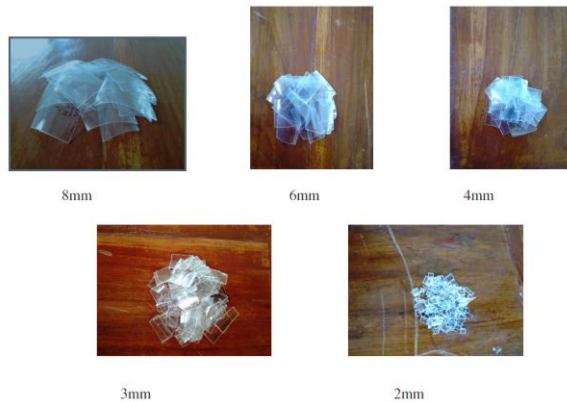
Figure 1: Different grain sizes of PET considered in the composite brick samples.
