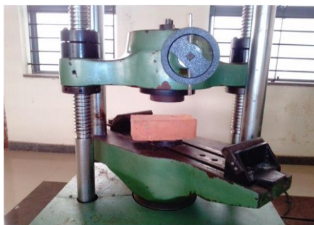
Figure 3: Testing of the composite bricks in Universal Testing machine
